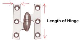
Order Templaco Router Template by Stock Number. Because of the small size of this hinge you must use a 3/8" outside diameter cutter with a 5/8" OD template guide or a 5/8" top mounted bearing on a 3/8" cutter. Order our TBK-1 top mounted bearing kit to use with your 3/8" cutter if you are not using a template guide.
